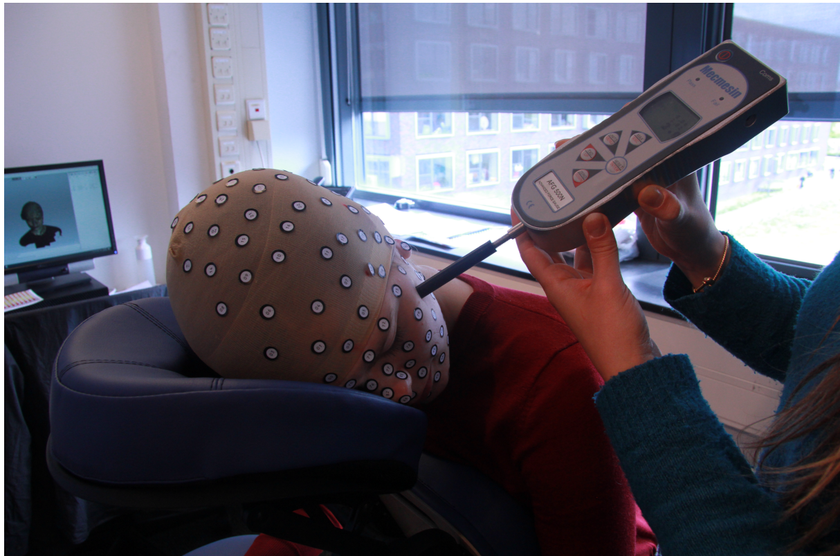
Figure 2 | Mecmesin AFG 500N pressure gauge with 3D printed PLA Ø10mm tip, and participant with EEG 10-20 landmark grid headcap and landmark stickers on the face, head and neck. Researcher gradually increasing pressure on a landmark with pressure gaug.
