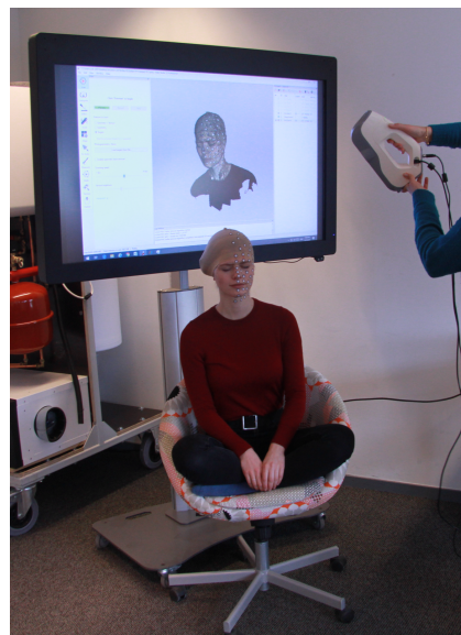
Figure 5 | 3D scanning the head, face and neck in order to capture the geometry and marker locations, using a rotating seat, Artec Eva 3D scanner and a reference monitor.
