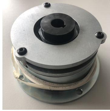
Figure 17: FSB035 electromagnetic brake
