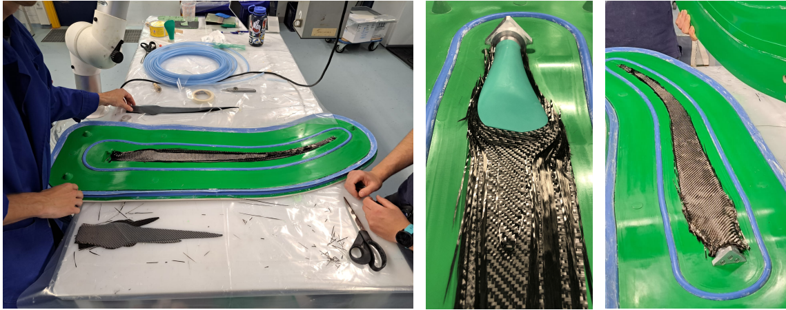
Figure 9: Carbon-fibre layup in the blade mould
