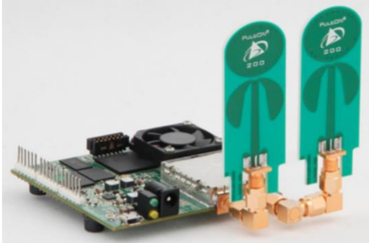
Figure 2: The PulsON P410 - Time Domain (Humatics) radar.
